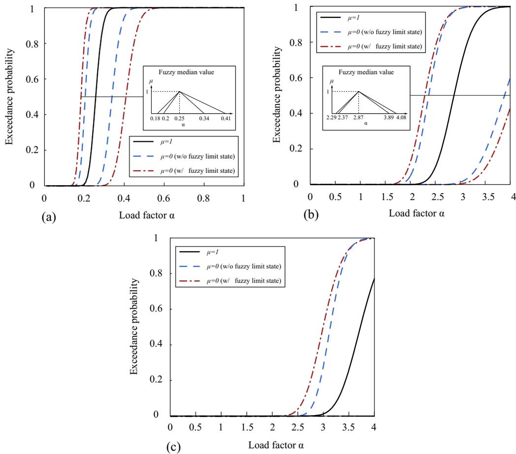
**FIGURE 8** Fragility curves of the model structure: (a) IO damage level; (b) LS damage level; and (c) CP damage level
