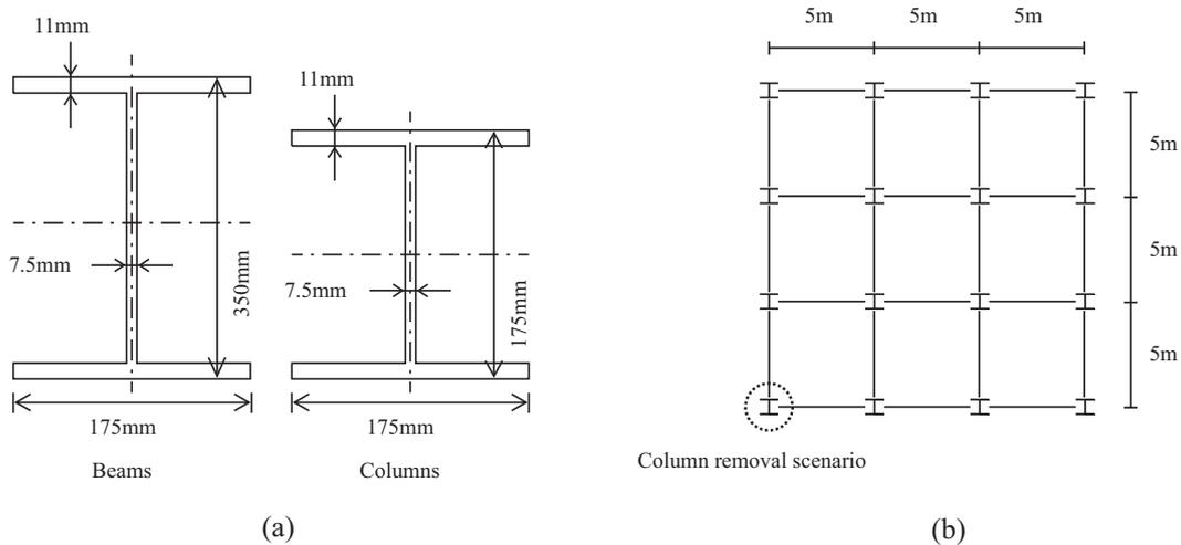
FIGURE 6 Details of the considered structure: (a) nominal dimensions of beam and column sections; (b) plan of the structure and the considered column removal scenario
