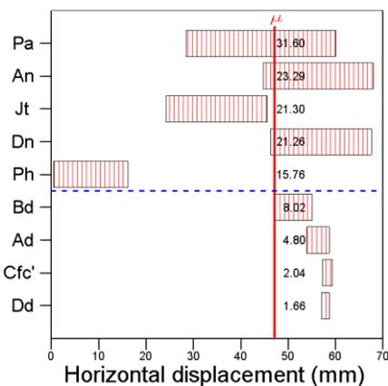
Fig. 10 Tornado diagram of displacement for various reinforcement methods
