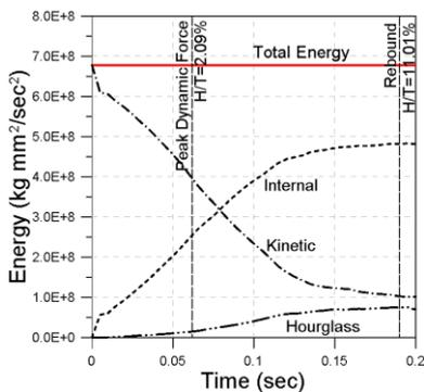
Fig. 3 Evolution of various energy quantities in the column subjected to the vehicle collision with impact speed of 30 km/h
