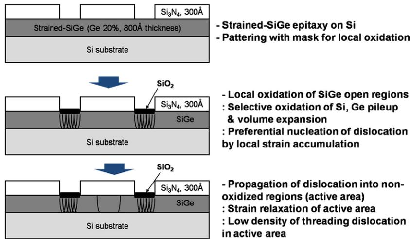
Fig. 1. Schematic illustration of local oxidation process for controlling dislocation positions in the SiGe buffer layer.
