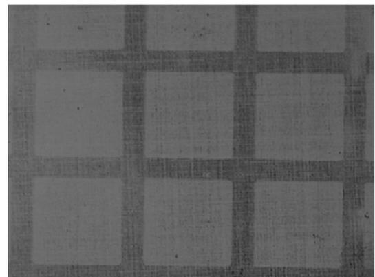
Fig. 3. Optical microscopy images of SiGe surface after removing  $\text{Si}_3\text{N}_4$  mask and  $\text{SiO}_2$  layer and Secco etching. The square pattern of the non-oxidized region has a size of  $200 \times 200 \mu\text{m}^2$ .
