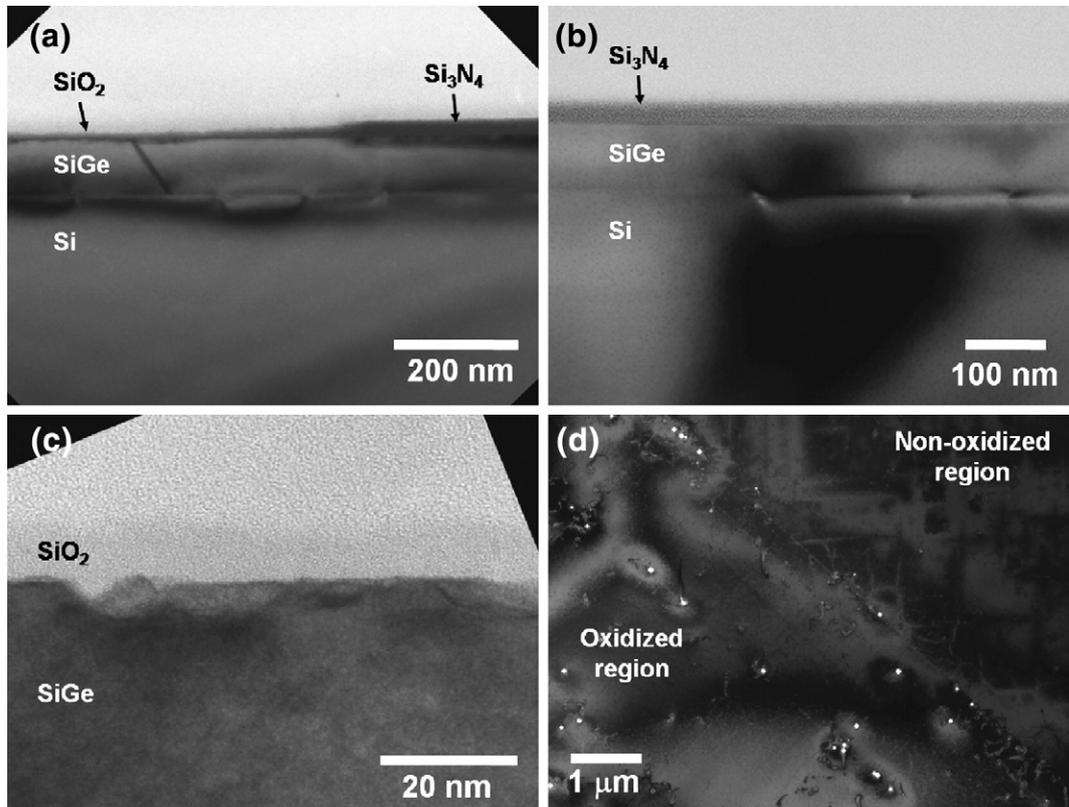
Fig. 5. Cross-sectional TEM images (a) showing both oxidized and non-oxidized SiGe layers, (b) magnified image of non-oxidized region and (c) oxidized region, and (d) plan-view image of both oxidized and non-oxidized SiGe surfaces after removing  $\text{Si}_3\text{N}_4$  mask and  $\text{SiO}_2$  layer.
