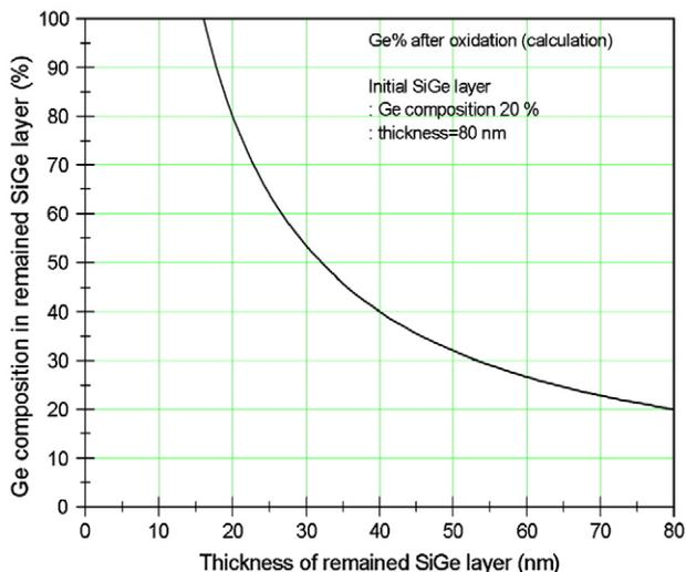
Fig. 2. Calculation of Ge composition as a function of the thickness of the remaining SiGe layer after oxidation.
