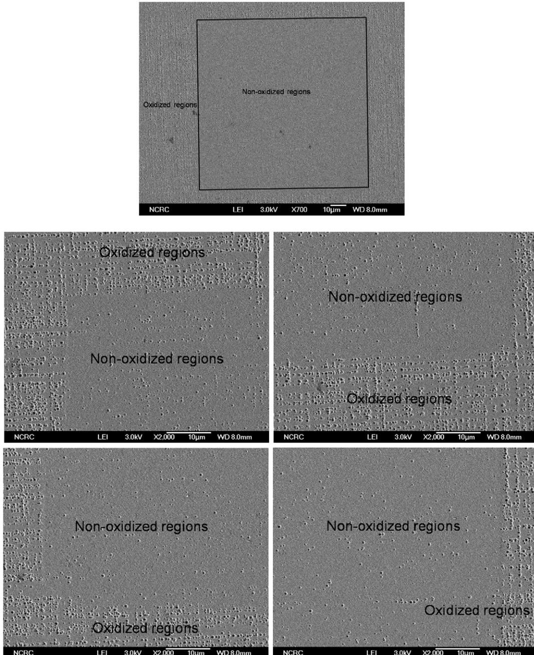
Fig. 4. SEM images of SiGe surface after removing  $\text{Si}_3\text{N}_4$  mask and  $\text{SiO}_2$  layer and Secco etching. The square pattern of the non-oxidized region has a size of  $100 \times 100 \mu\text{m}^2$ .
