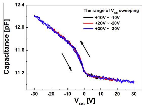
Fig. 2. The  $C$ – $V$  characteristic of the organic memory without CdSe NPs. (PMMA/PMMA insulator).
