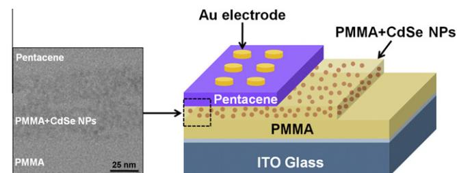
Fig. 1. Schematic illustration of memory architectures and cross-sectional TEM image of the fabricated device featuring CdSe NPs embedded in PMMA layer.
