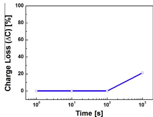
**Fig. 4.** Retention characteristics in terms of the charge loss ( $\Delta C$ ) after applying  $-30$  V gate stress voltage for 1 s.
