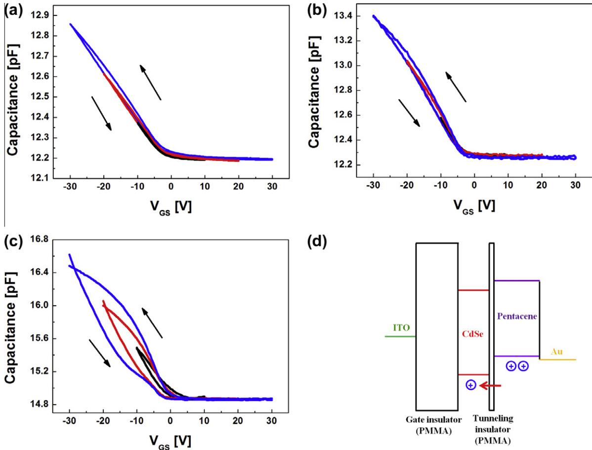
**Fig. 3.** The C–V characteristic of the fabricated organic memory with different concentrations of CdSe NPs at different  $V_{GS}$  sweeping range, (a)  $7.3 \times 10^{14}$ , (b)  $1.0 \times 10^{15}$ , (c)  $2.0 \times 10^{15}$  particles/ml. (d) Schematic illustration of the energy band structure of the organic memory without CdSe NPs.
