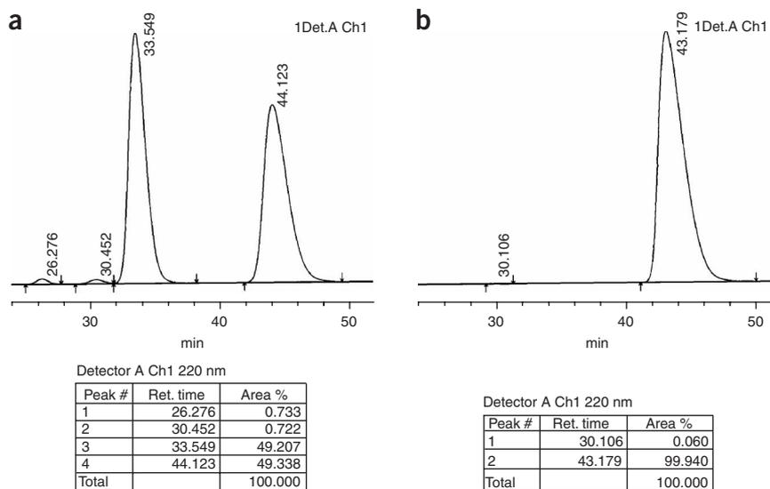
**Figure 4** | HPLC chromatograms. (a) The racemic compound and (b) the enantiopure compound (Chiralpak AS-H column, 2% *i*-PrOH/heptane, 0.50 ml min<sup>-1</sup>, 220 nm).
