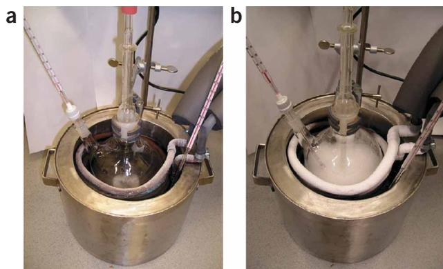
**Figure 2** | The reaction setup of hexanal with benzaldehyde-derived *N*-Boc-imine **2a** in the presence of (*S*)-Pro (20 mol%) in acetonitrile. (a) Reaction mixture after mixing all compounds. (b) Reaction mixture after completion the reaction (24 h). Boc, *tert*-butoxycarbonyl.
