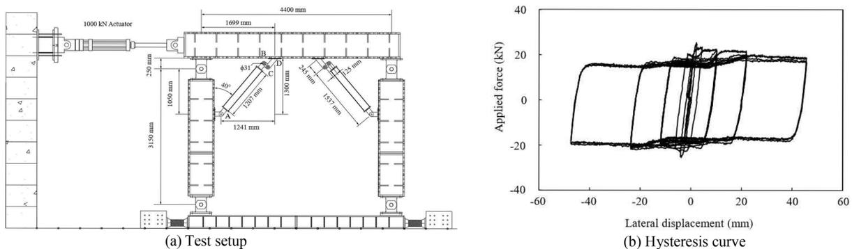
**Figure 2.** Cyclic loading test of the corner rotational friction dampers.
