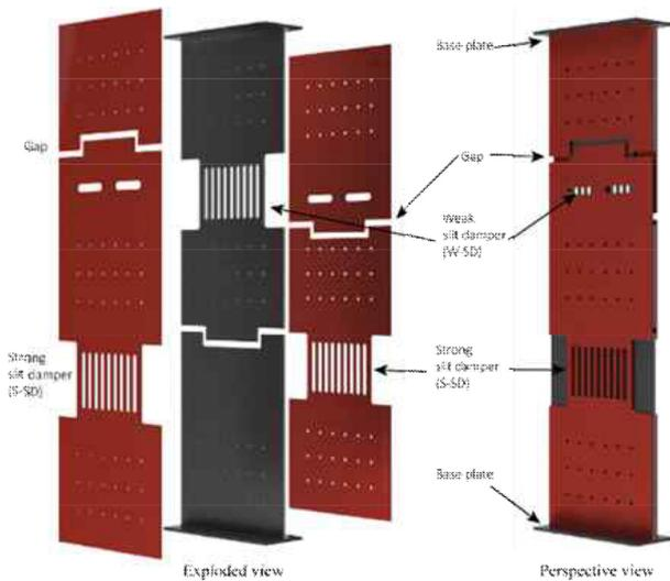
Figure 6. Multi-slit damper.
