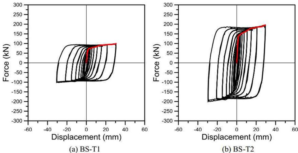
Figure 5. Hysteresis curves of the test specimens.
