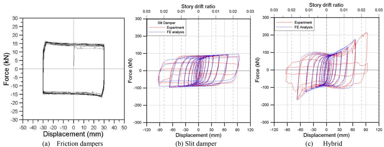
Figure 10. Hysteresis curves of the damper obtained from cyclic loading test.
