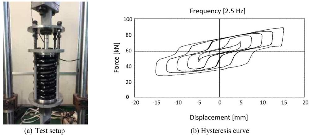
Figure 11. Loading test of the spring-viscous damper.
