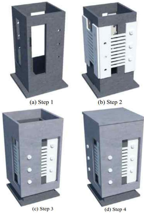
Figure 3. Assembly of the damper.
