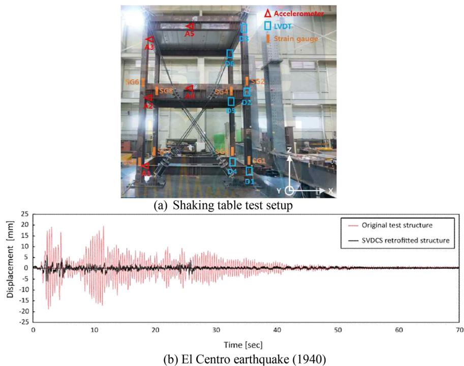
Figure 12. Shaking table test of the spring-viscous damper cable system.
