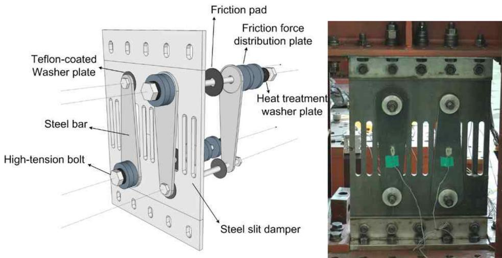
Figure 9. Hybrid slit-friction damper.
