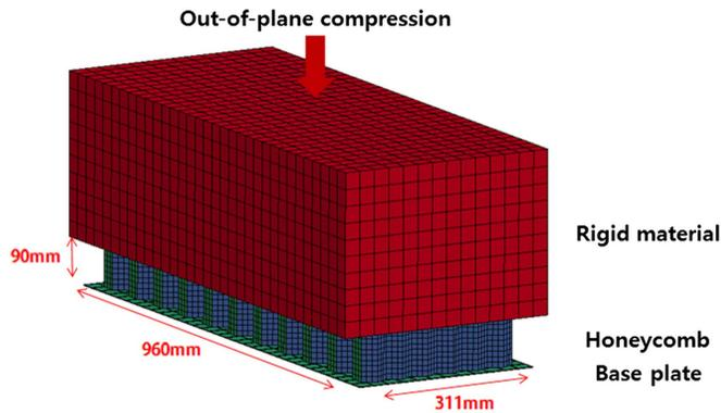
Fig. 8. Out-of-plane impact analysis of the honeycomb panel.
