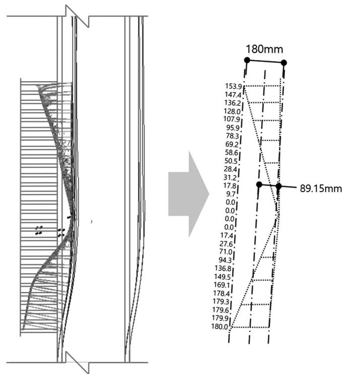
**Fig. 14.** Mean deformation of the honeycomb panel after the truck collision.
