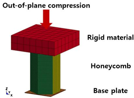
Fig. 3. Impact simulation of the honeycomb structure.
