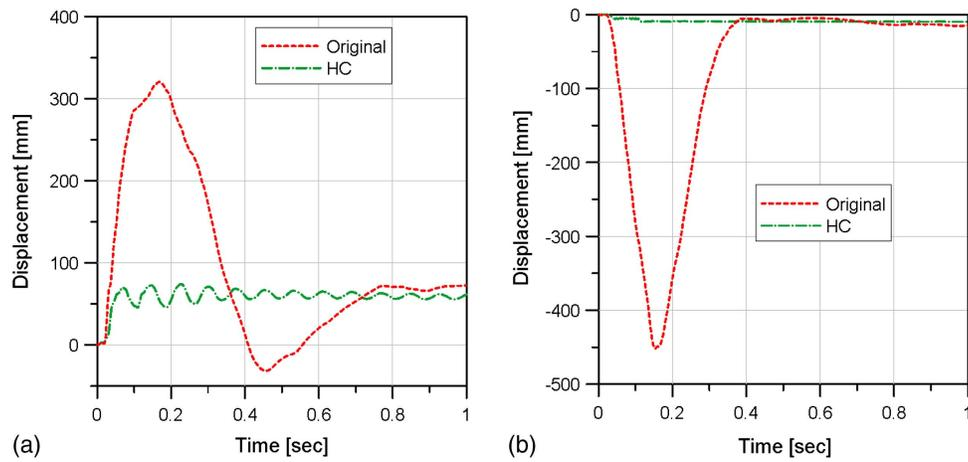
**Fig. 13.** Displacement time histories of the column due to the truck collision: (a) horizontal displacement; and (b) vertical displacement.
