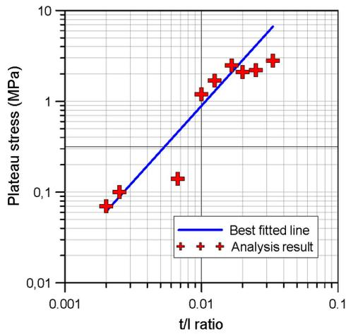
**Fig. 6.** Relationship of  $t/l$  ratio and static plateau stress.
