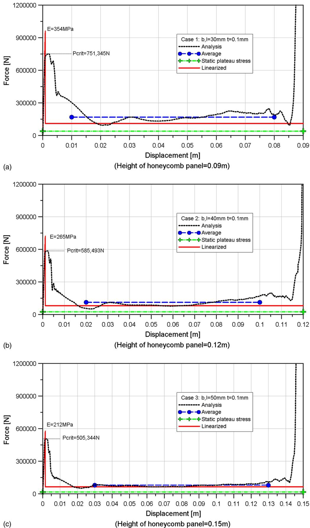
**Fig. 10.** Stress-strain relationship of the honeycomb panel under compression with  $t = 0.1$  mm: (a)  $b = 30$  mm; (b)  $b = 40$  mm; and (c)  $b = 50$  mm.
