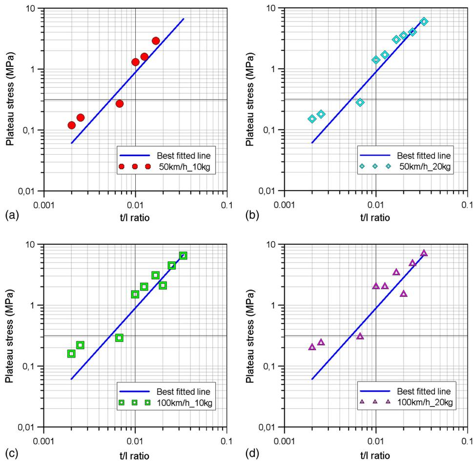
**Fig. 7.** Relationship of  $t/l$  ratio and dynamic plateau stress: (a) impact velocity = 13 m/s and mass of impactor = 10 kg; (b) impact velocity = 13 m/s and mass of impactor = 20 kg; (c) impact velocity = 27 m/s and mass of impactor = 10 kg; and (d) impact velocity = 27 m/s and mass of impactor = 20 kg.
