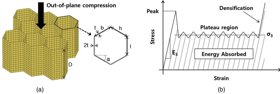
**Fig. 1.** Mechanical properties of a honeycomb cell: (a) geometry of hexagonal honeycomb cell; and (b) out-of-plane stress-strain behavior of honeycomb under compression.
