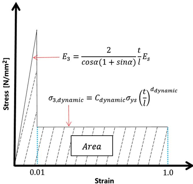
Fig. 9. Linearized stress-strain curve of honeycomb panel.
