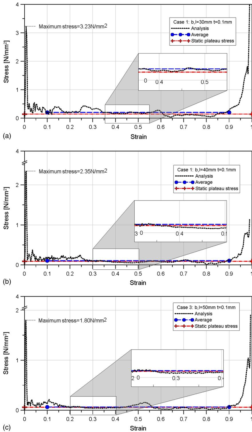
**Fig. 5.** Stress-strain relationship of a single honeycomb cell under compression with  $t = 0.1$  mm: (a)  $b = 30$  mm; (b)  $b = 40$  mm; and (c)  $b = 50$  mm.
