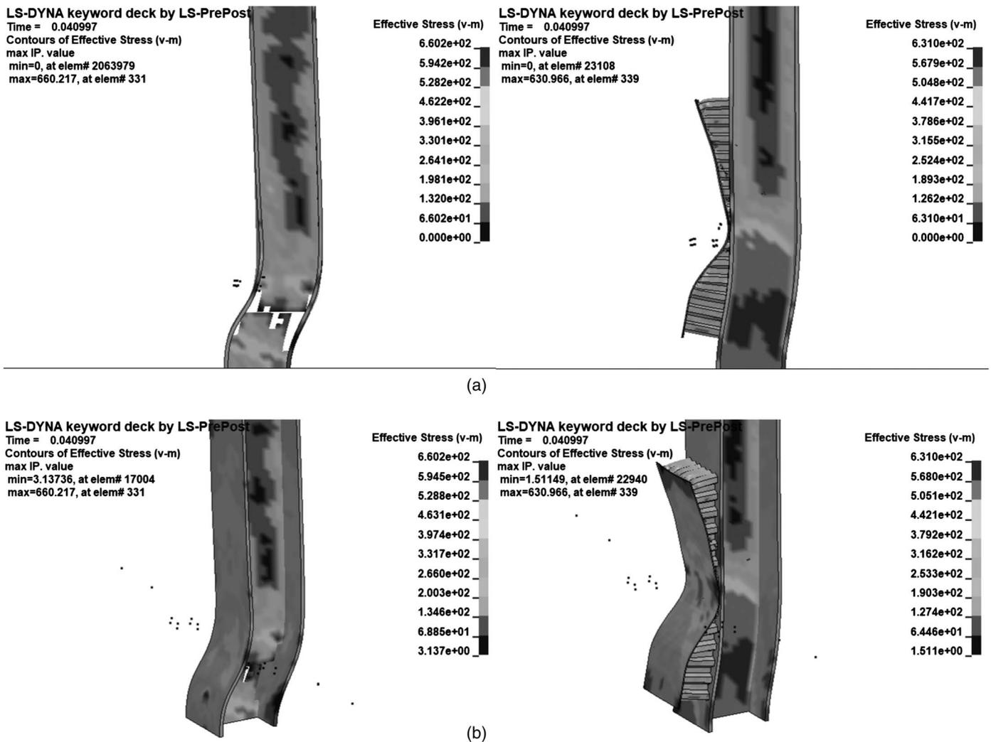
**Fig. 12.** Stress distribution at damaged column with honeycomb panel ( $t = 0.4$  s): (a) side view; and (b) three-dimensional view.
