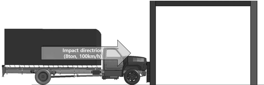
**Fig. 11.** Truck collision analysis of a simple frame.
