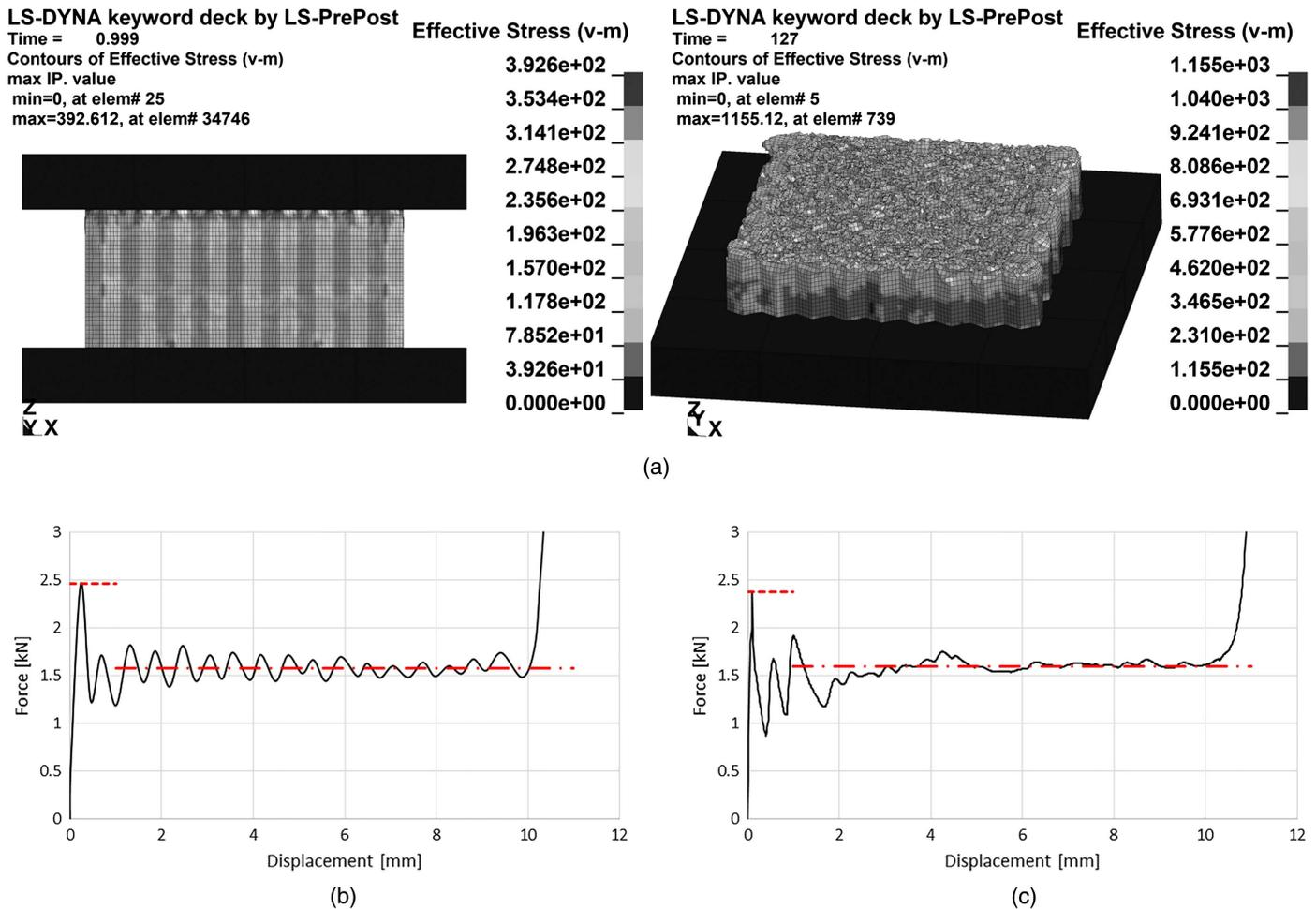
**Fig. 2.** Comparison of the impact test results obtained by Xu et al. (2012) and numerical analysis results: (a) LS-DYNA FE numerical model of the test specimen; (b) experimental result (Xu et al. 2012); and (c) FE analysis result of the test specimen.
