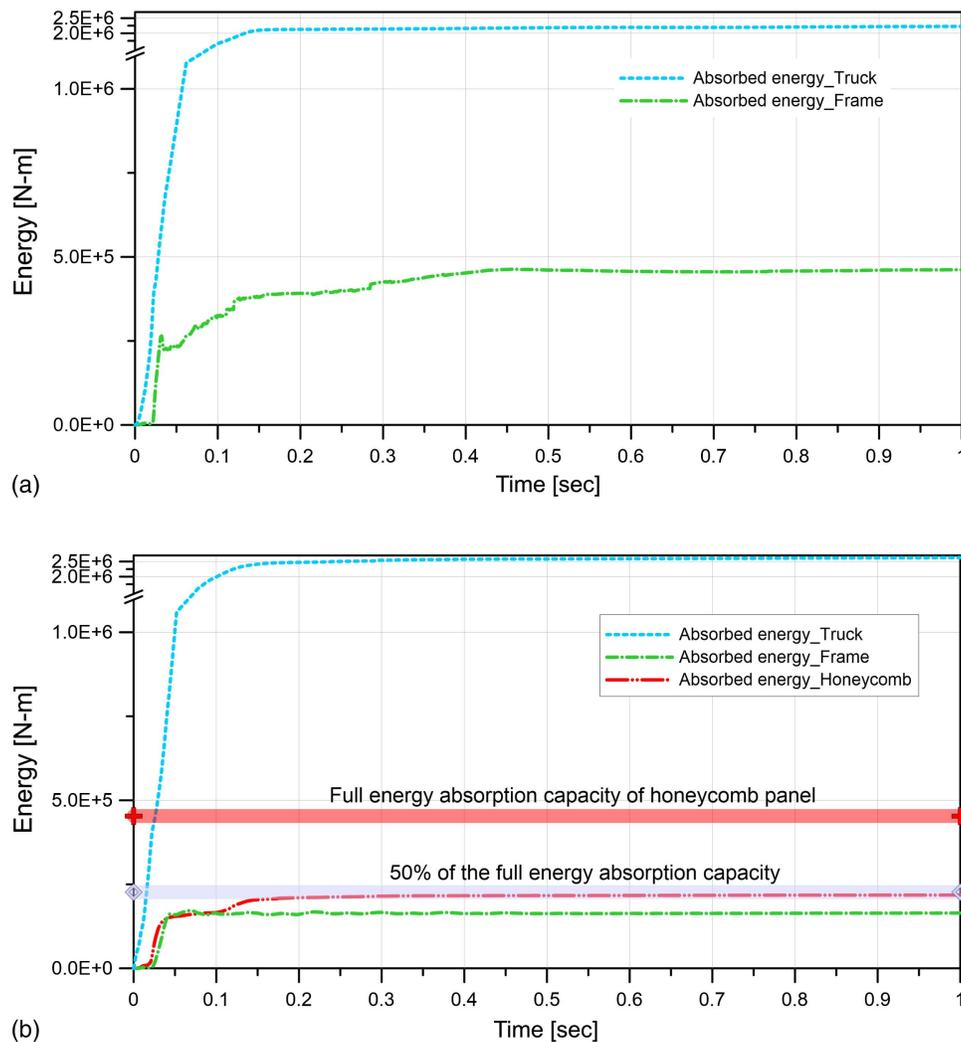
**Fig. 15.** Time history of the impact energy caused by the truck collision: (a) time history of the bare frame; and (b) time history of the installed frame.
