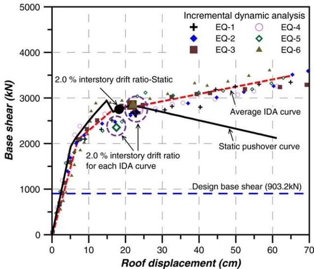
Fig. 20. Static and dynamic pushover curves of the six-story SCBF.
