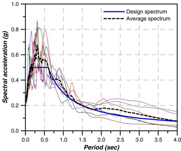
Fig. 19. Design spectrum and response spectra of selected earthquake records.
