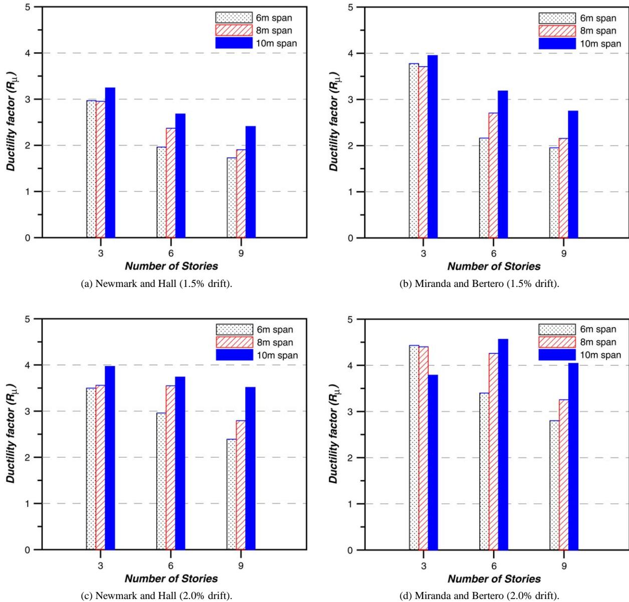
Fig. 15. System ductility factors of OCBFs.
