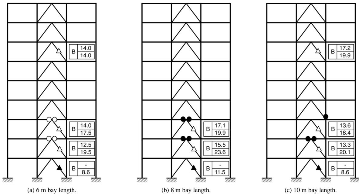
Fig. 9. Location of inelastic deformation and brace ductility ratios of the nine-story OCBFs.
