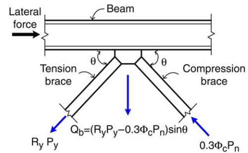
Fig. 3. Unbalanced force due to buckling of compression brace.
