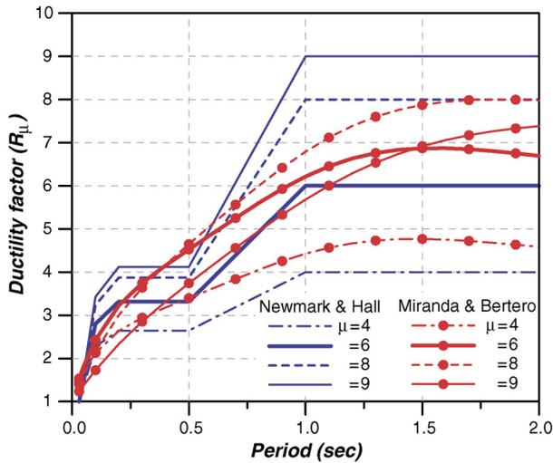
Fig. 16. Comparison of ductility factors computed from Newmark and Hall and Miranda and Bertero’s equations.
