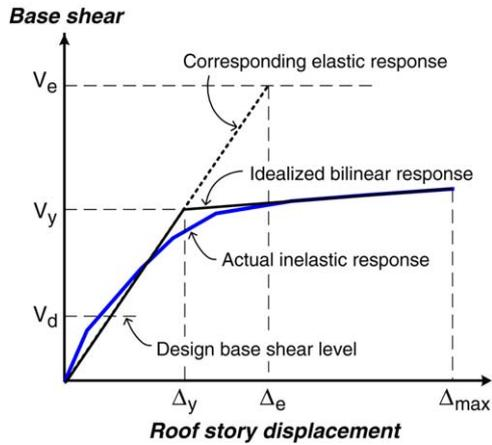
Fig. 1. Lateral load–roof displacement relationship of a structure.
