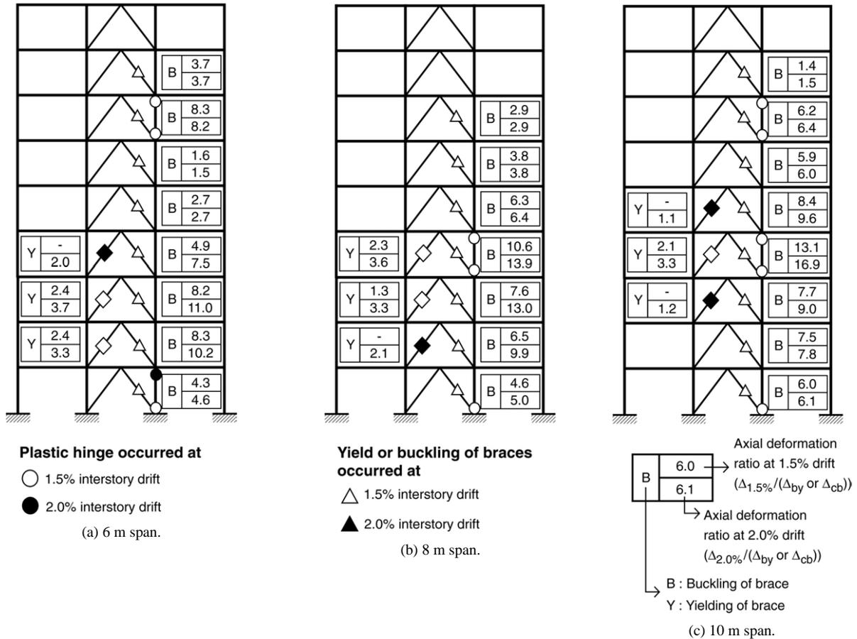
Fig. 8. Locations of inelastic deformation and brace ductility ratios of the nine-story SCBFs.
