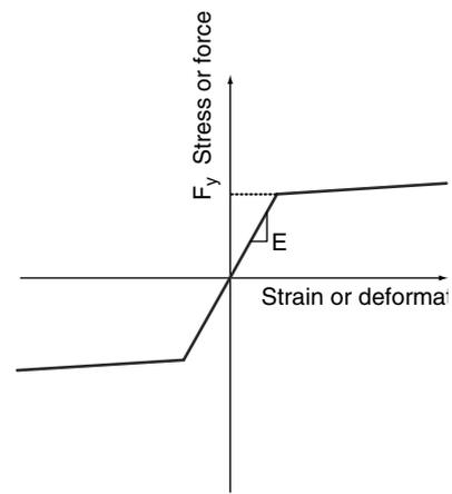
Figure 1. Material modeling for steel members (Steel01)
