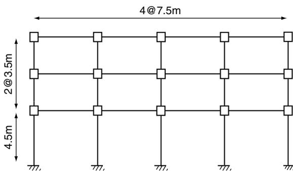
**Figure 6.** Side-view of 3-storey model structure
