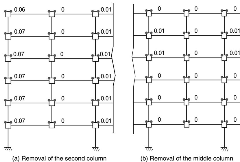
**Figure 16.** Maximum plastic rotations of panel zones of 6-storey GLRS structure
