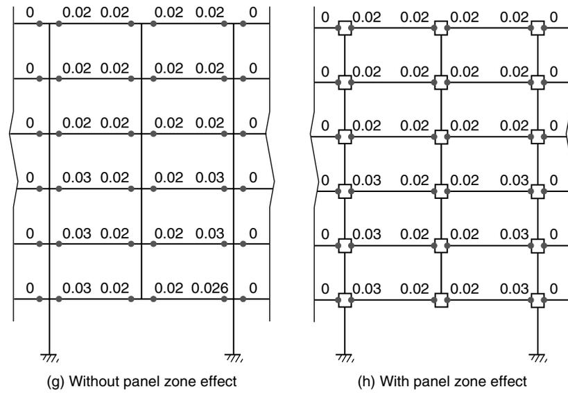
Figure 14. Maximum plastic rotations of beams in 6-storey GLRS structure caused by removal of the middle column
