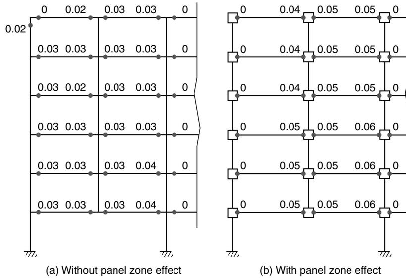
Figure 13. Maximum plastic rotations of beams in 6-storey GLRS structure caused by removal of the second column
