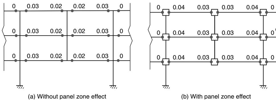
**Figure 12.** Maximum plastic rotations of beams in 3-storey GLRS structure caused by removal of the middle column
