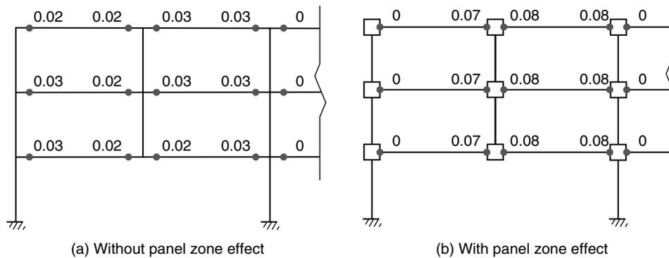
**Figure 11.** Maximum plastic rotations of beams in 3-storey GLRS structure caused by removal of the second column
