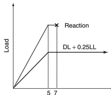
**Figure 8.** Application of vertical load for dynamic analysis
