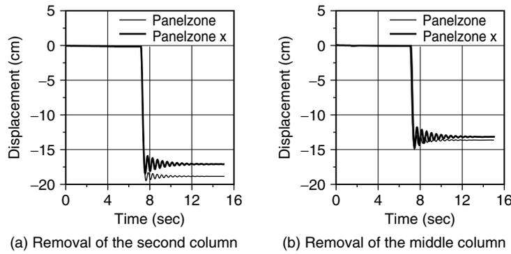
Figure 18. Nonlinear dynamic analysis results of 6-storey LLRS
