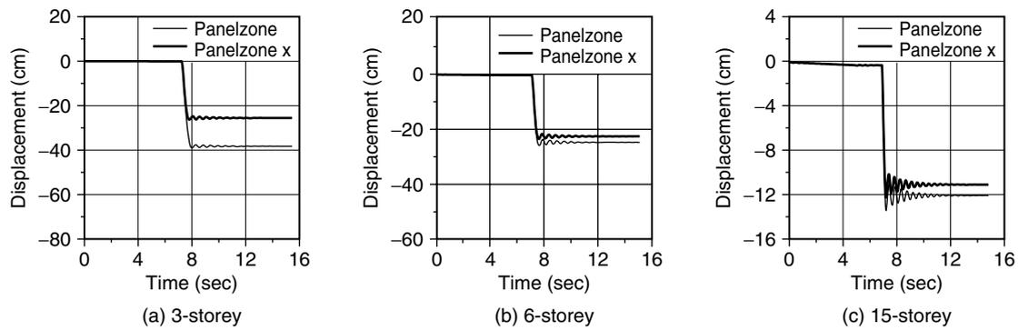
**Figure 10.** Nonlinear dynamic analysis results of the GLRS model structures with the middle column removed
