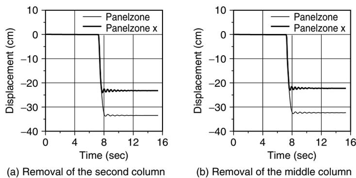
**Figure 17.** Nonlinear dynamic analysis results of 3-storey LLRS
