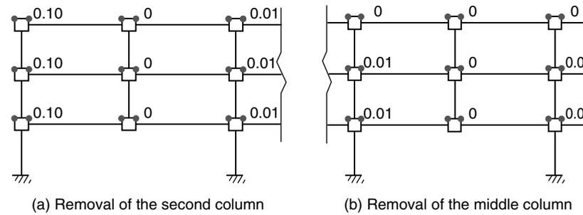
Figure 15. Maximum plastic rotations of panel zones of 3-storey GLRS structure
