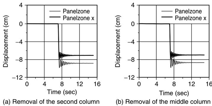
Figure 19. Nonlinear dynamic analysis results of 15-storey LLRS
