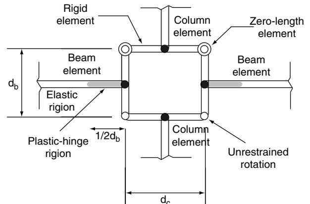
Figure 2. Modeling of beam-column joint with panel zone (Gupta and Krawinkler 1999)
