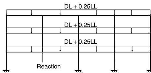
**Figure 7.** Gravity loads for progressive collapse analysis
