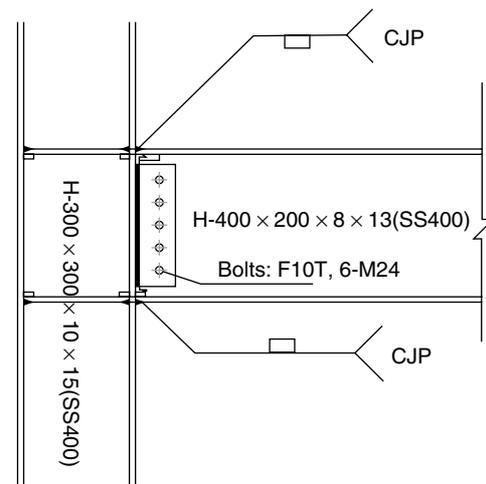
Figure 3. Specimen for monotonic loading test (Kim *et al.* 2007)
