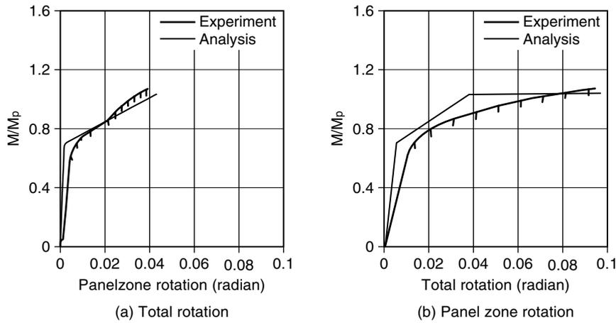
Figure 4. Comparison of moment-rotation relationships of steel joint obtained from analysis model and experiment
