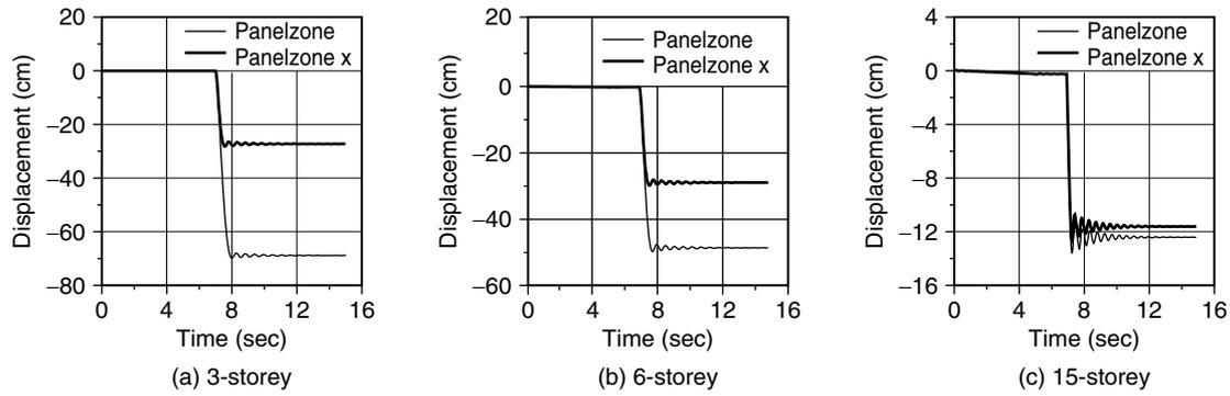
Figure 9. Nonlinear dynamic analysis results of the GLRS model structures with the second column removed
