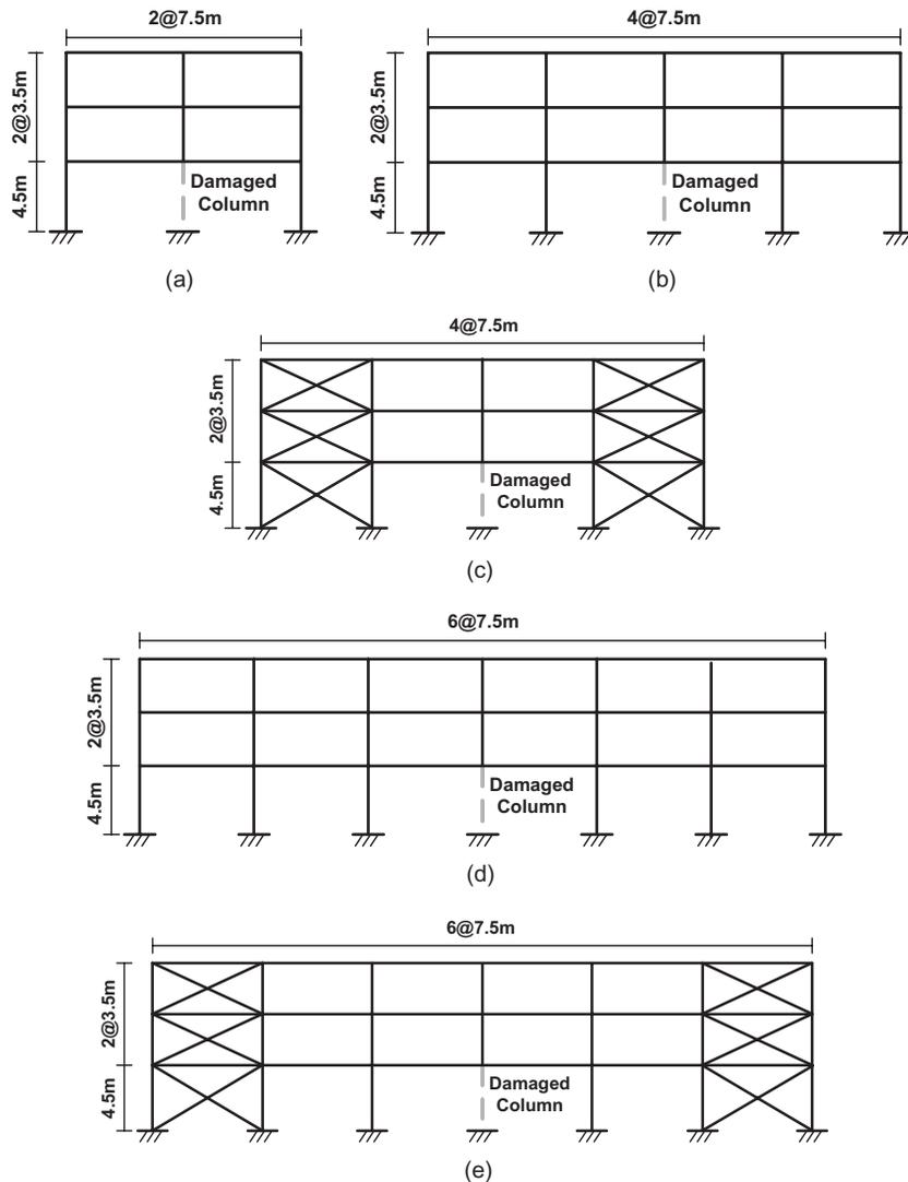
Figure 6. Three-story analysis model structures. (a) Two-bay model. (b) Four-bay model. (c) Four-bay model with braces. (d) Six-bay model. (e) Six-bay model with braces
