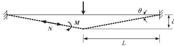
Figure 1. Definition of rotation angle in a beam model
