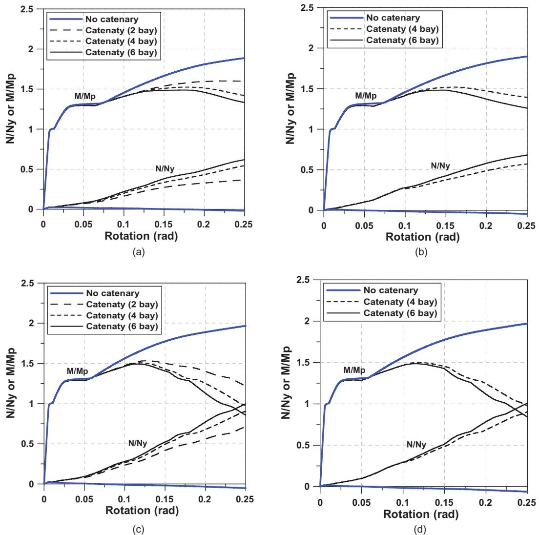
Figure 7. Variation of axial force and bending moment of model structures obtained from push-down analysis. (a) Three-story models without braces. (b) Three-story models with braces. (c) Six-story models without braces. (d) Six-story models with braces
