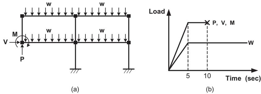
Figure 4. Imposed loads for progressive collapse. (a) Loading on a structure with a column remove. (b) Time history of loads
