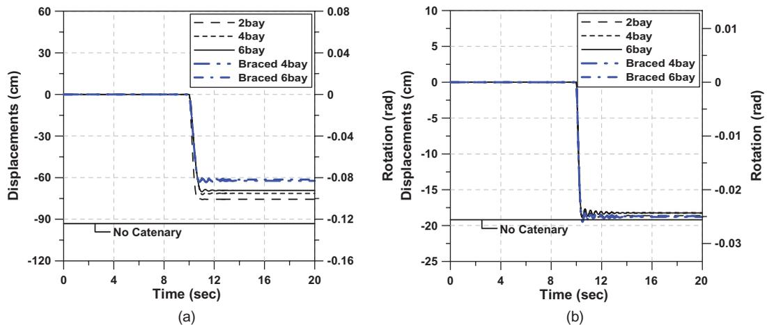
Figure 9. Displacement time histories of model structures obtained from non-linear dynamic analysis. (a) Three-story structures. (b) Six-story structures
