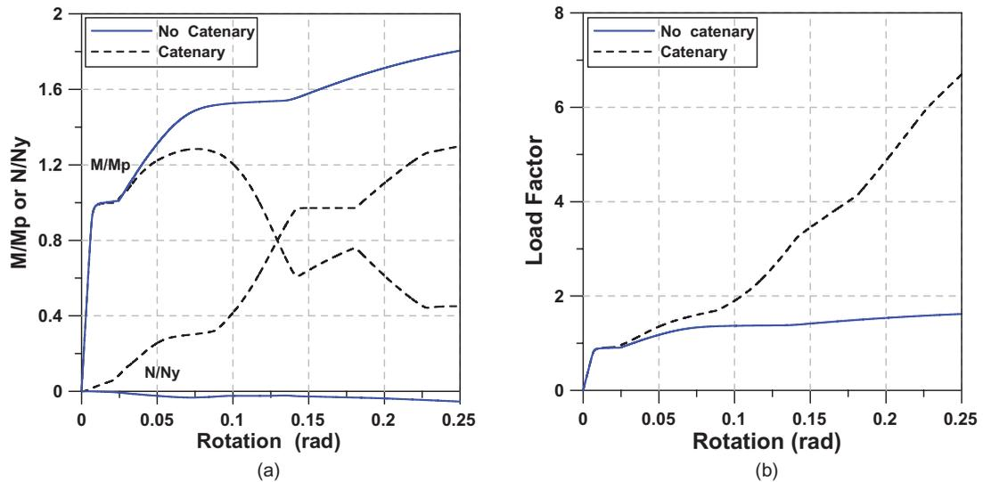
Figure 3. Push-down analysis results of the simple model. (a) Variation of member forces. (b) Push-down curves
