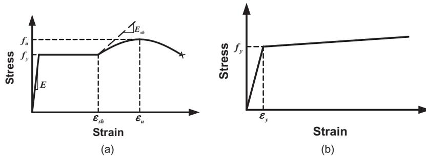
Figure 2. Non-linear material models used in the analysis. (a) Steel 01 model for columns and braces. (b) Reinforcing steel model
