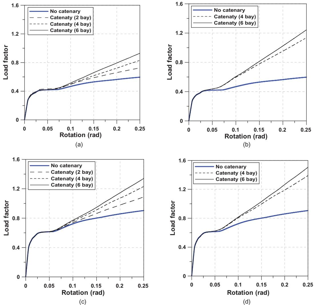
Figure 8. Push-down curves of the model structures with and without considering catenary action. (a) Three-story models without braces. (b) Three-story models with braces. (c) Six-story models without braces. (d) Six-story models with braces
