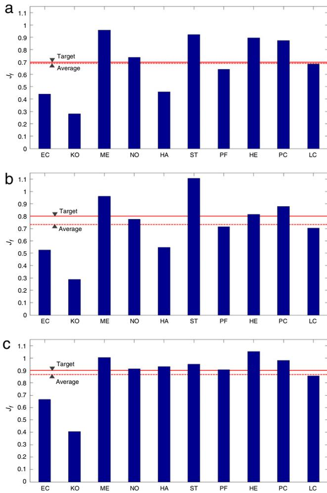
**Fig. 14.** Response reduction factors for a single-story structure with  $f_n = 0.5$  Hz. (a) Target response reduction factor  $J_f = 0.7$ . (b) Target response reduction factor  $J_f = 0.8$ . (c) Target response reduction factor  $J_f = 0.9$ .
