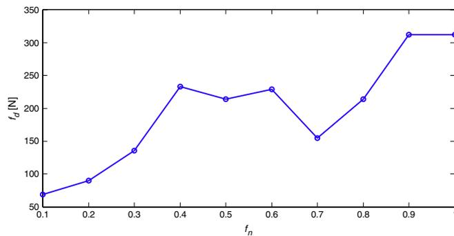
Fig. 12. Designed friction damper forces for a single-story structure with various  $f_n$ 's and  $J_f = 0.8$  under the El Centro earthquake.
