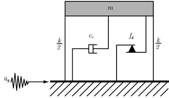
Fig. 1. A single-story structure installed with a friction damper subjected to an earthquake load.
