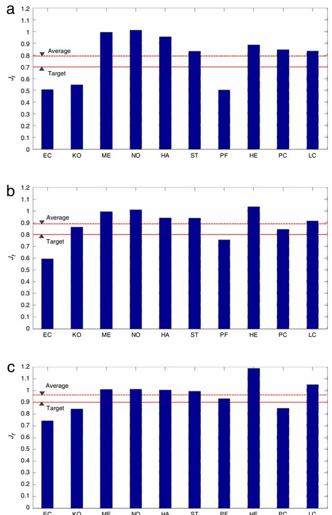
**Fig. 15.** Response reduction factors for a single-story structure with  $f_n = 0.8$  Hz. (a) Target response reduction factor  $J_f = 0.7$ . (b) Target response reduction factor  $J_f = 0.8$ . (c) Target response reduction factor  $J_f = 0.9$ .
