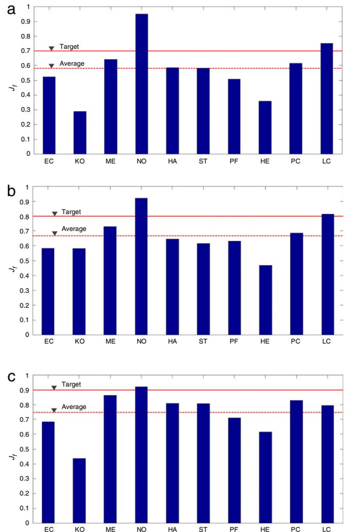
Fig. 13. Response reduction factors for a single-story structure with  $f_n = 0.2$  Hz. (a) Target response reduction factor  $J_f = 0.7$ . (b) Target response reduction factor  $J_f = 0.8$ . (c) Target response reduction factor  $J_f = 0.9$ .
