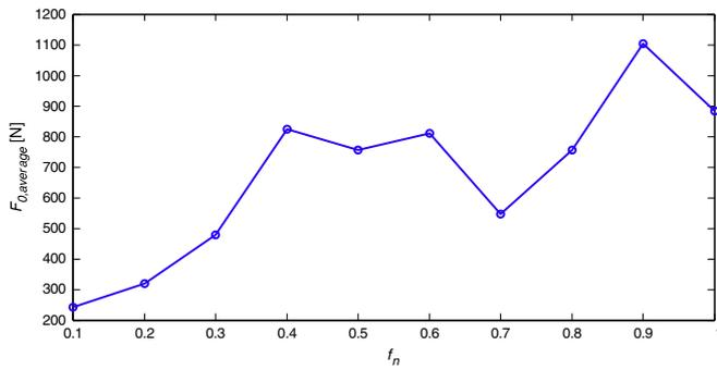
Fig. 10.  $F_{0,average}$  for a single-story structure with various  $f_n$ 's under the El Centro earthquake.
