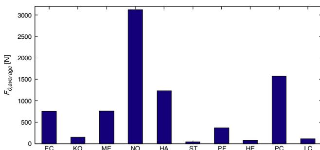
Fig. 9.  $F_{0,\text{average}}$  for a single-story structure with  $f_n = 0.5$  Hz under 10 seismic records.
