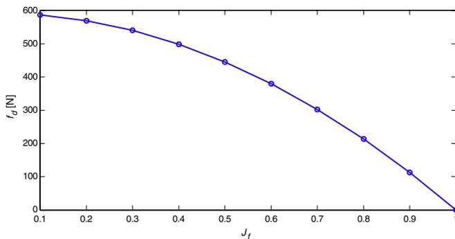
Fig. 11. Designed friction damper forces for a single-story structure with  $f_n = 0.5$  Hz under the El Centro earthquake.
