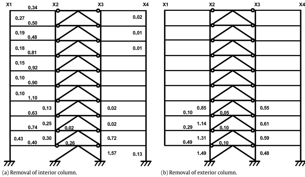
Fig. 19. Coefficient of variability of the dual system building to uncertain member strengths.
