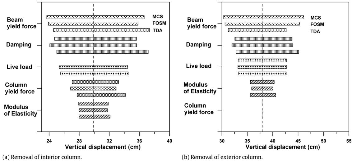
Fig. 11. Vertical displacement sensitivity of the three-story building: dynamic analysis.
