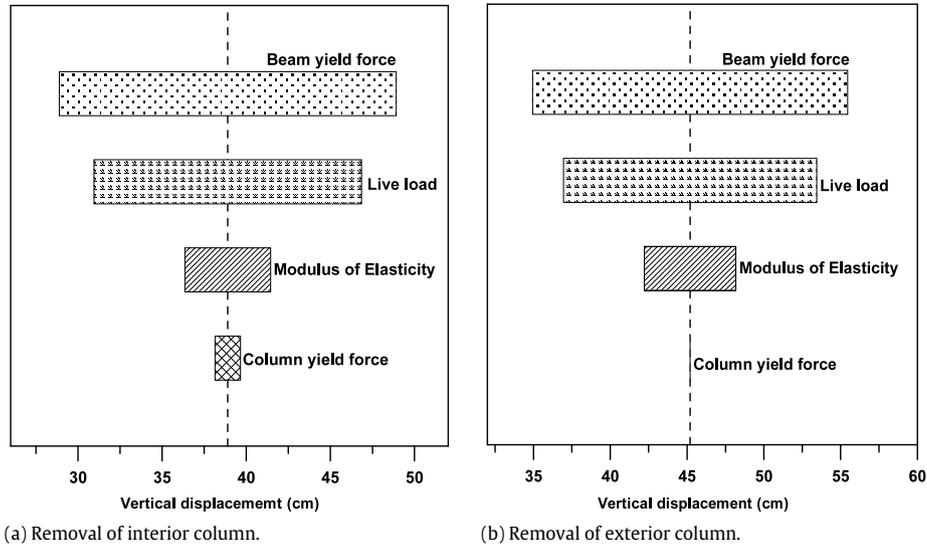
Fig. 14. Vertical displacement sensitivity of the ten-story moment-resisting frame building: static analysis.
