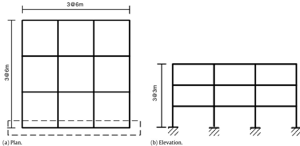
Fig. 5. Plan and elevation of the three-story case study building.
