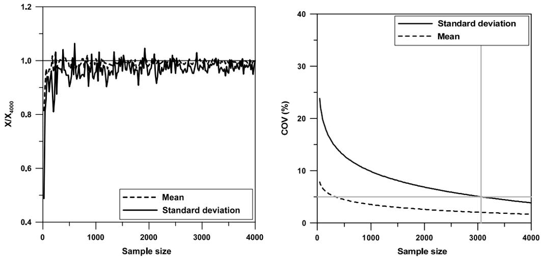
Fig. 9. Convergence test of MCS for dynamic analysis.
