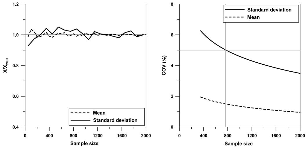
Fig. 8. Convergence test of MCS for static analysis.
