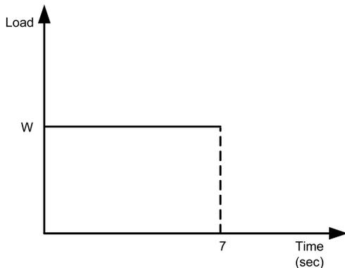
Fig. 3. Applied load for dynamic progressive collapse analysis.
