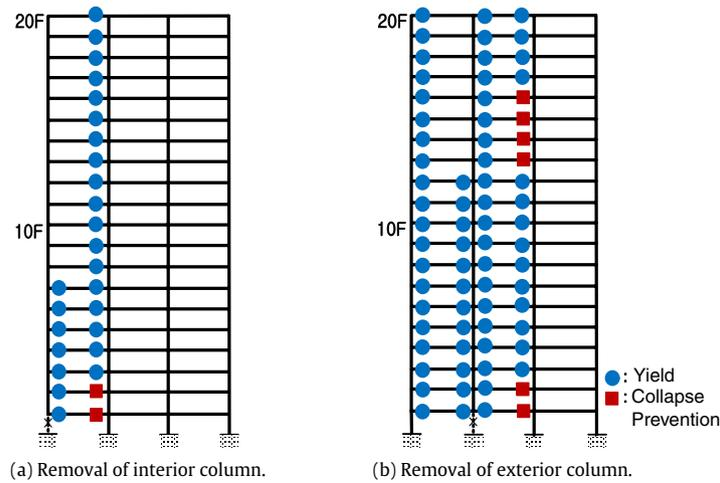
Fig. 22. Plastic hinge rotation at beam ends.
