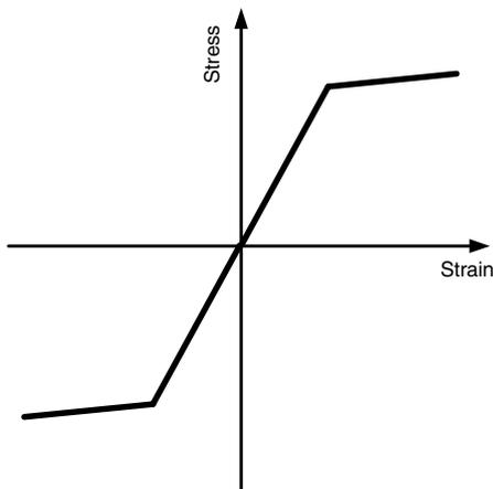
Fig. 6. Stress–strain relationship of the Steel01 material model of OpenSees.
