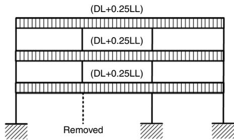
Fig. 2. Load combination for structural analyses.
