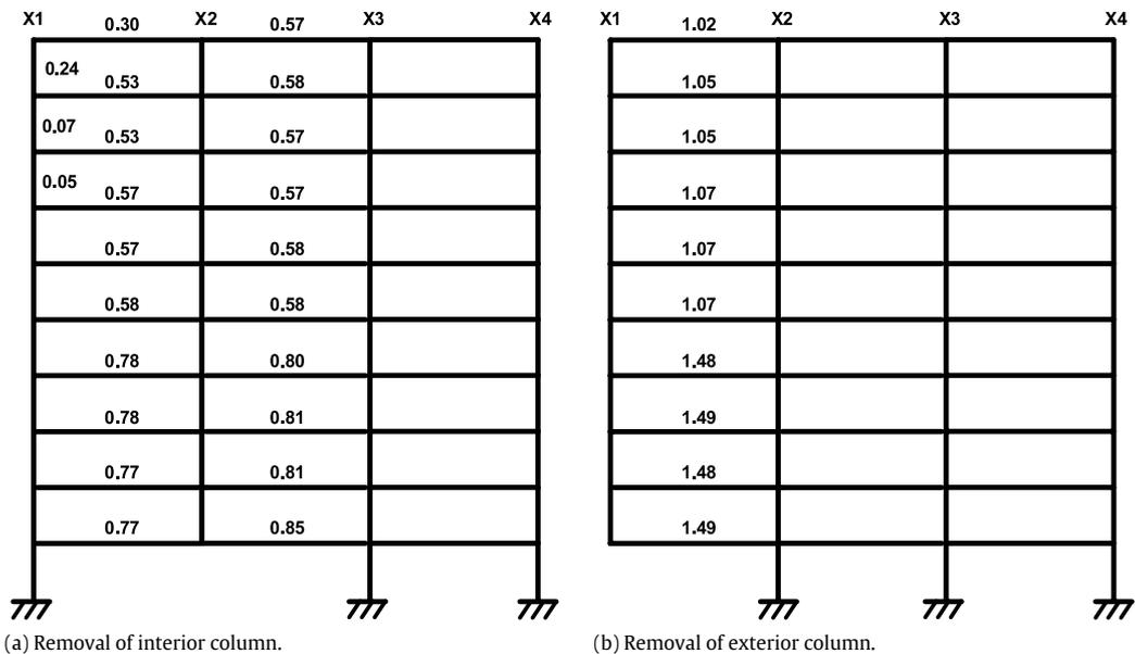
Fig. 18. Coefficient of variability of the moment-resisting frame to uncertain member strengths.
