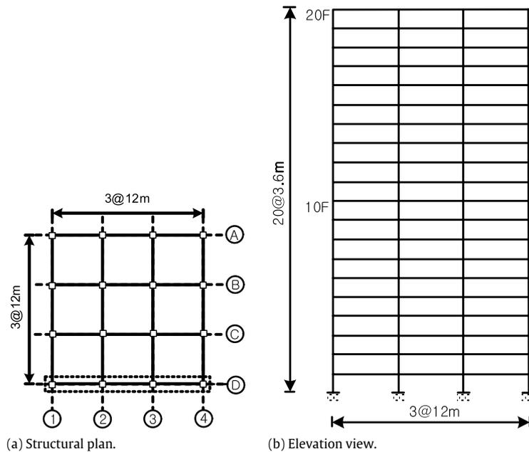
Fig. 20. Twenty-story analysis model structure.
