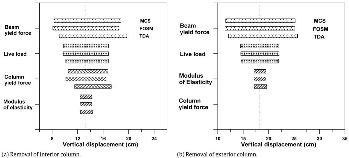
Fig. 10. Vertical displacement sensitivity of the three-story building: static analysis.
