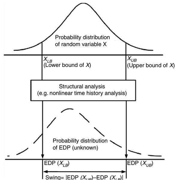
Fig. 4. Tornado diagram analysis procedure [17].
