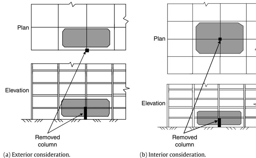
Fig. 1. Allowable collapse zone [7].
