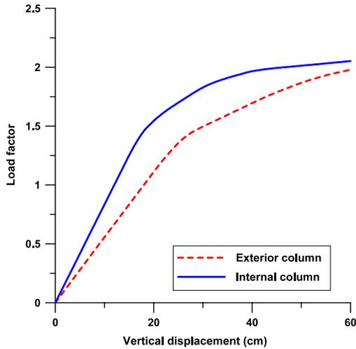
Fig. 21. Force-vertical displacement relationship when a first-story column is removed.
