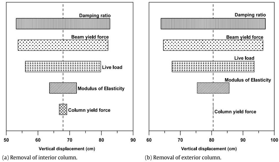
Fig. 15. Vertical displacement sensitivity of the ten-story moment-resisting frame building: dynamic analysis.
