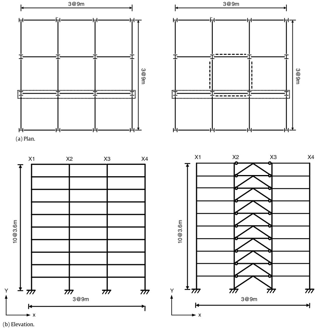
Fig. 12. Plan and elevation view of the ten-story case study buildings.
