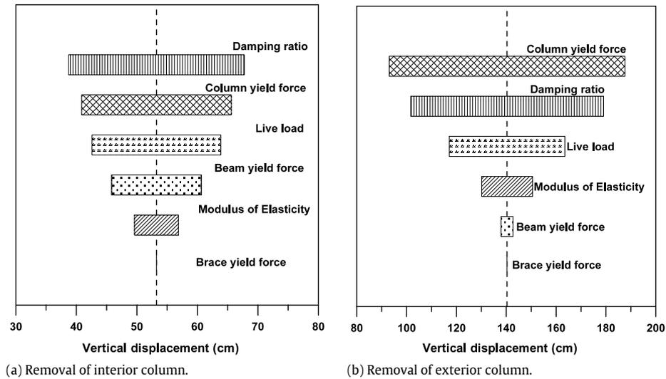
Fig. 17. Vertical displacement sensitivity of the ten-story dual system building: dynamic analysis.
