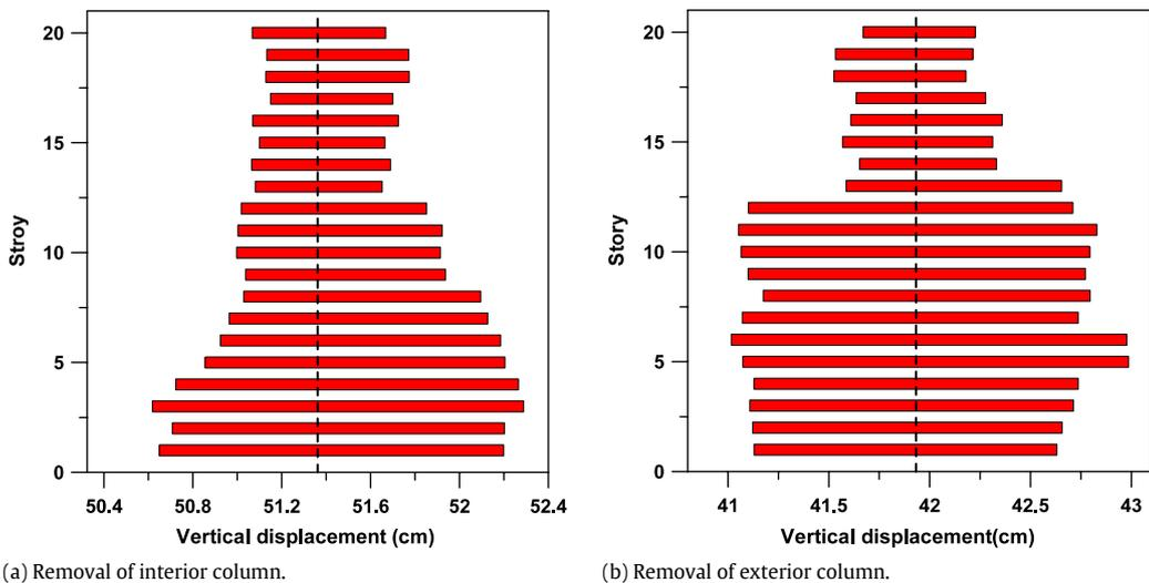
Fig. 23. Variation of vertical displacement at exterior bay due to variation of beam yield strength at collapse prevention limit state.
