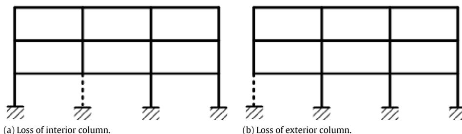
Fig. 7. Two cases of initial conditions for collapse analysis.
