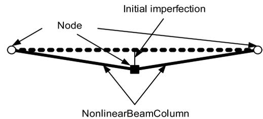
Fig. 13. Modeling of the bracing members.
