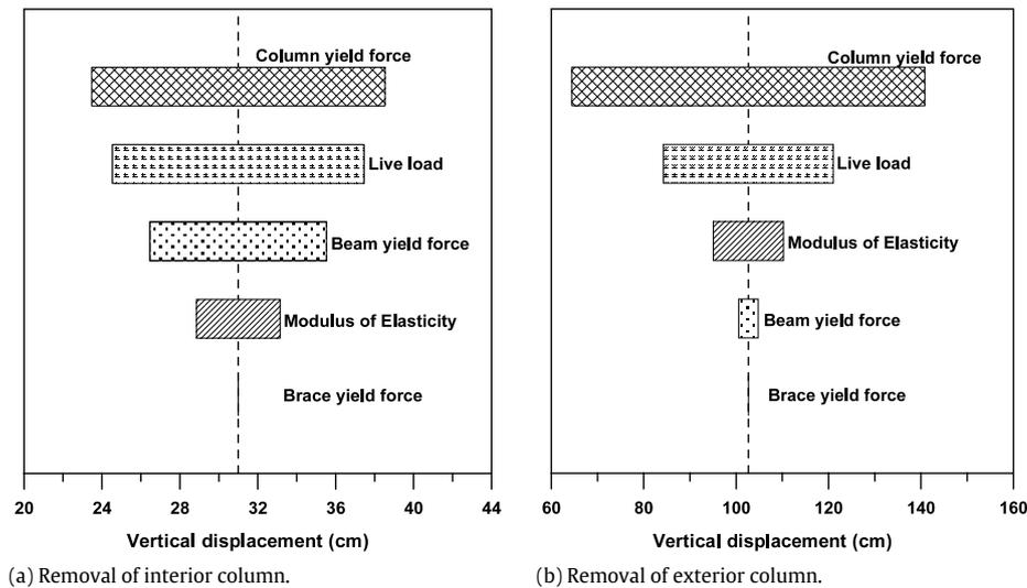
Fig. 16. Vertical displacement sensitivity of the ten-story dual system building: static analysis.
