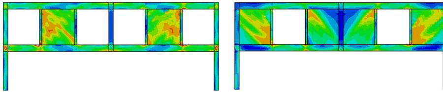
Fig. 7. Distribution of stress at partial steel plates when vertical displacement reached 100 mm.
