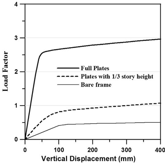
Fig. 8. Pushdown curves of the two-story frame installed with partial steel plates with 1/3 of story height.
