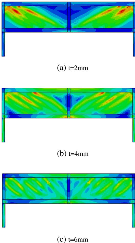
Fig. 5. Von-Mises stress contours in the infill steel plate when the vertical displacement reached 50 mm.
