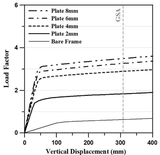
Fig. 4. Pushdown curves of the two-story 9 m span model structure with full infill panels.
