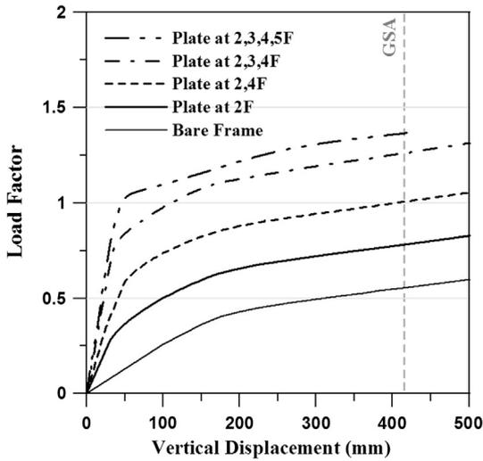
Fig. 11. Pushdown curves of five-story model with and without steel plates.
