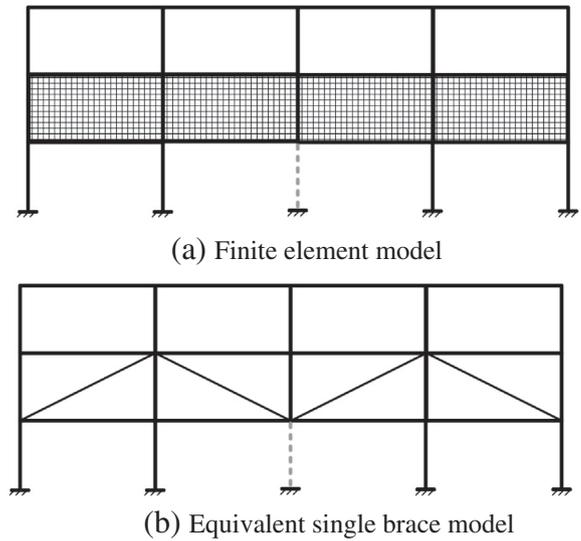
Fig. 16. Configuration of three-story analysis model structure with infill panels for validation of simplified modeling of infill steel panels.
