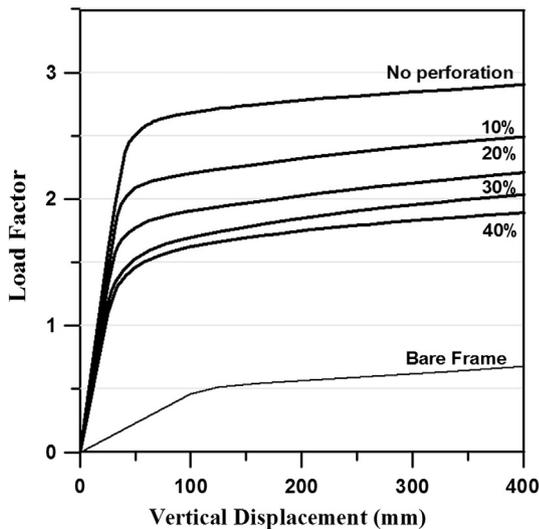
Fig. 9. Pushdown curves of the two-story structure with 4 mm thick infill plates with various perforation rates.
