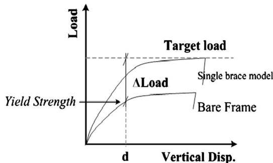
Fig. 15. Target strength of the frame for design of infill steel panels.
