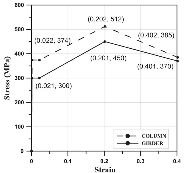
Fig. 2. Idealized stress-strain relationship for structural steel.
