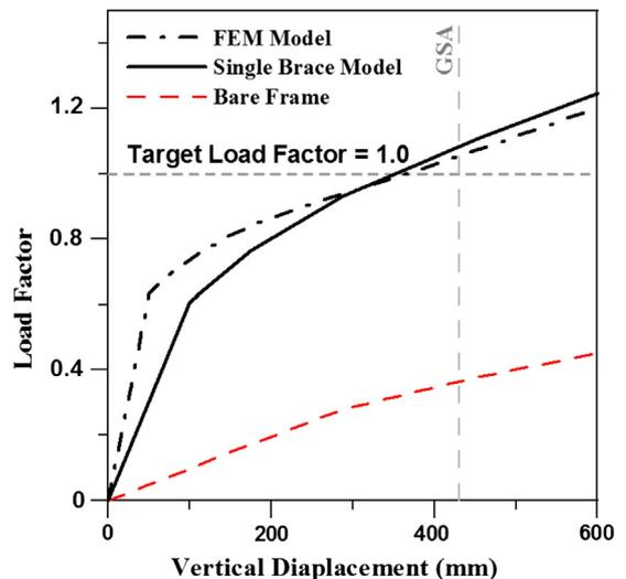
Fig. 17. Pushdown curves of the three-story model structure with infill plates designed using Eq. (6).
