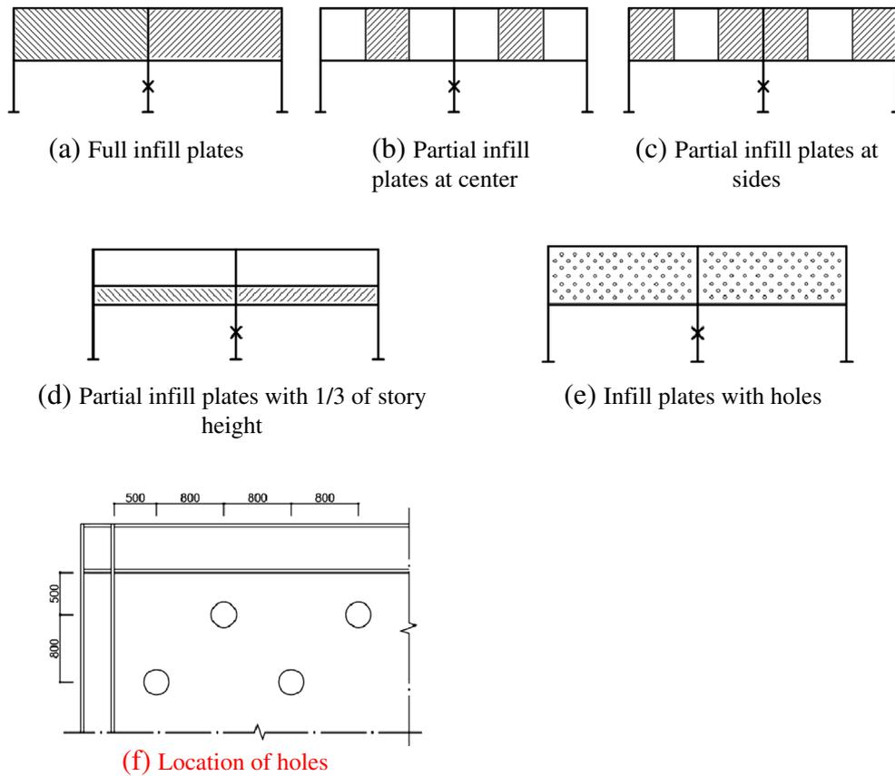
Fig. 3. Configuration of infill steel panels used in the analysis.
