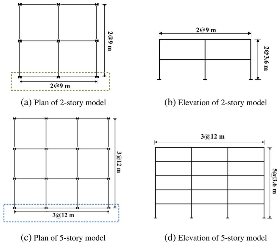
Fig. 1. Structural plan and elevation of analysis model structures.
