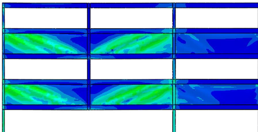
Fig. 12. Von-Mises stress contours in the five-story structure at vertical displacement of 100 mm.
