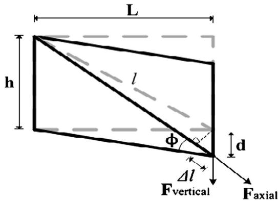
Fig. 14. Relation of vertical deflection and element force of an equivalent single brace.
