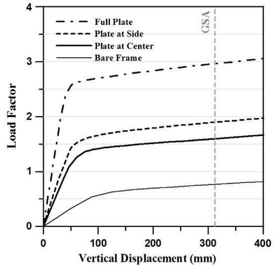
Fig. 6. Pushdown curves of the two-story 9 m span model structure with 4 mm thick partial infill panels.
