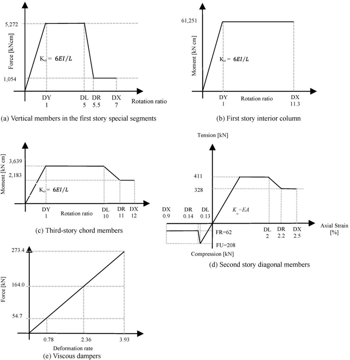
Fig. 5. Nonlinear force-displacement relationships of selected structural elements.
