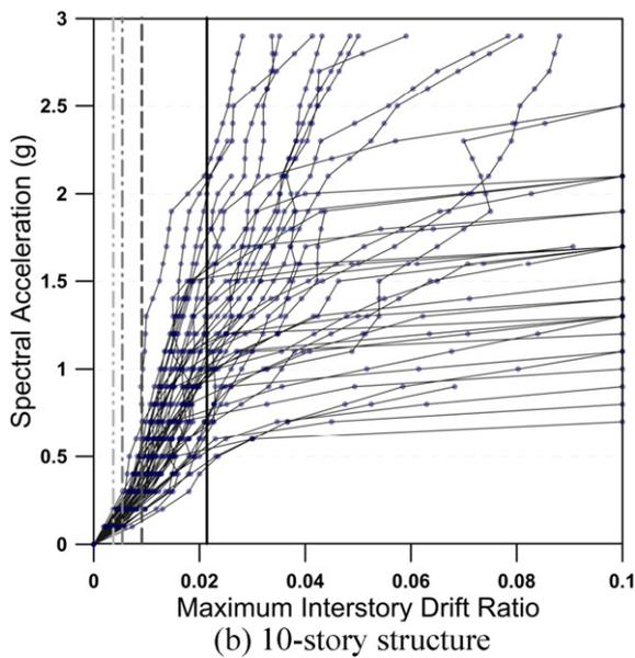
Fig. 20. Incremental dynamic analysis results of the structures with viscous dampers.
