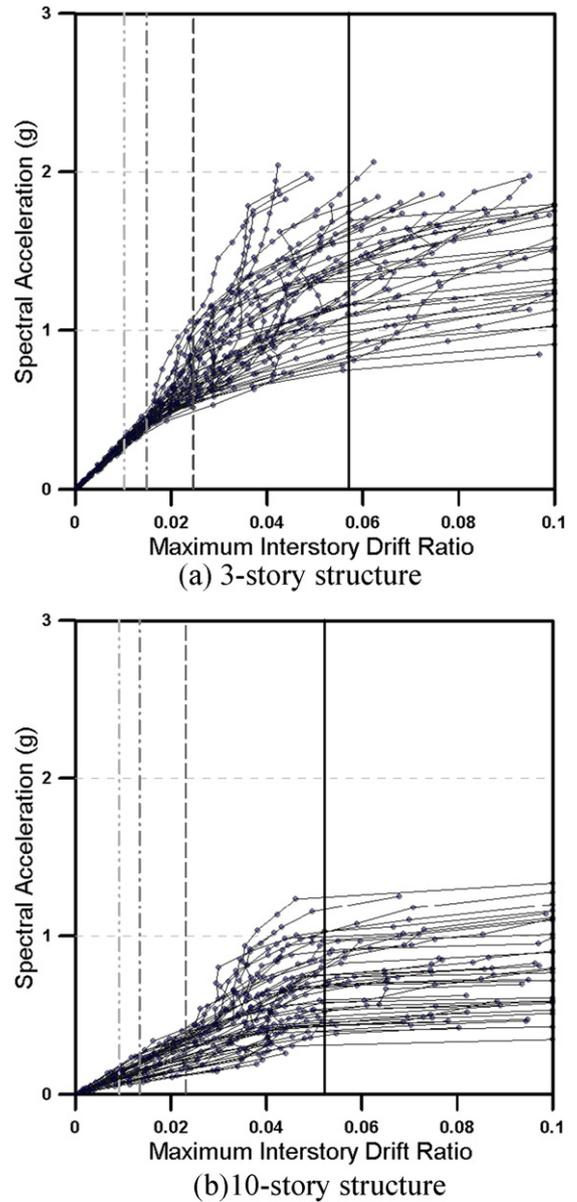
Fig. 10. Incremental dynamic analysis results of SMRF structures.
