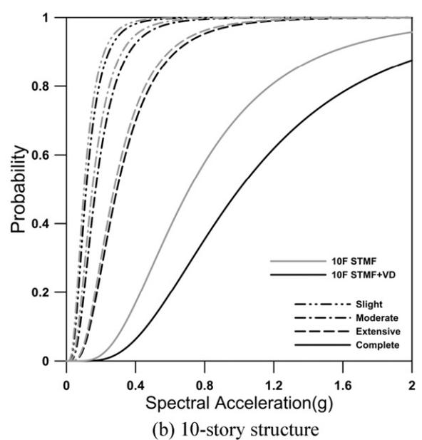
Fig. 21. Comparison of fragility curves of the model structures with and without viscous dampers.
