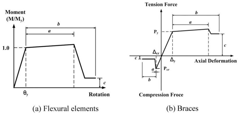
Fig. 4. Nonlinear force-displacement relationships of structural elements.
