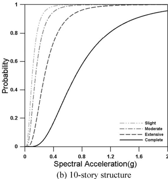
Fig. 11. Fragility curves of STMF model structures.
