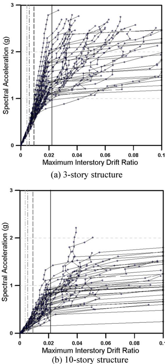
Fig. 9. Incremental dynamic analysis results of STMF structures.
