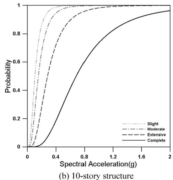
Fig. 12. Fragility curves of SMRF model structures.
