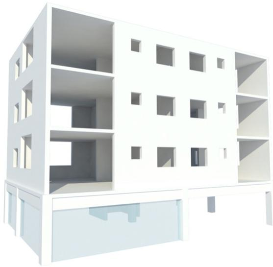
Fig. 24. Perspective view of the 4-story structure with plan and vertical asymmetry.
