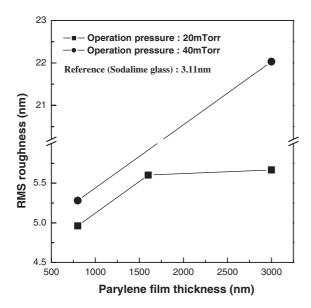
Fig. 5. RMS roughness of the parylene films deposited on a sodalime glass (the roughness of 3.11 nm) as a function of the deposition thickness and operation pressure measured by an AFM.
