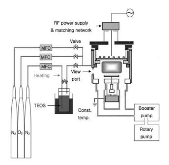
Fig. 1. Schematic diagram of the SiO<sub>2</sub> PECVD system used in the experiment.
