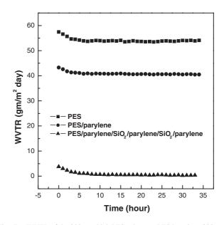
Fig. 7. WVTR of the  $300\,\mu m$  thick PES substrate, PES/parylene( $800\,n m$ ), and PES/parylene( $800\,n m$ )/SiO<sub>2</sub>( $100\,n m$ )/parylene( $800\,n m$ )/SiO<sub>2</sub>( $100\,n m$ )/parylene( $800\,n m$ ).
