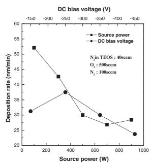
Fig. 2. Deposition rate of the  $SiO_2$  films by PECVD at low temperatures as a function of the source power and dc bias voltage. (condition:  $N_2$  in TEOS 40 sccm,  $O_2$  flow rate 500 sccm, and  $N_2$  flow rate 100 sccm)
