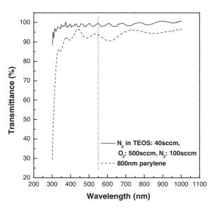
Fig. 6. Optical transmittance of the SiO<sub>2</sub> films deposited by PECVD on a sodalime glass substrate (condition: N<sub>2</sub> in TEOS 40 sccm, O<sub>2</sub> flow rate 500 sccm, N<sub>2</sub> flow rate 100 sccm, source power 500 W, and dc bias voltage –350 V) and the parylene films (800 nm, 20 mTorr) measured by a UV spectrometer. The vertical dash-dotted line indicates a wavelength of 550 nm, which was used as the wavelength for measuring the optical transmittance.
